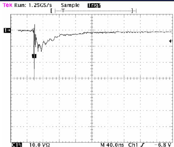
Figure 2. ESD Clamping Voltage Screenshot
