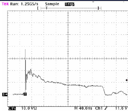
Figure 1. ESD Clamping Voltage Screenshot
